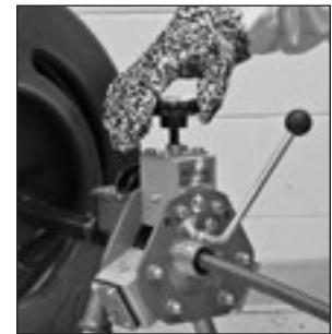
**DO NOT** run cable fittings (i.e. couplings, splicers, cable ends) through a tightened down auto feed. It can break feed wheels. Release the feed, pull fittings through manually and then re-engage.
