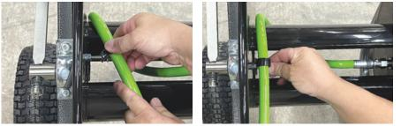
Position the clamp over the hose (with the flatter side next to the reel) and slide it on to the bolt. Finger tighten the nut.
