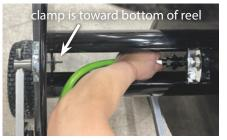
Remove the clamp and nut. Attach the hose to the opening which is opposite of the clamp side. Use a wrench to make sure it is secure.
