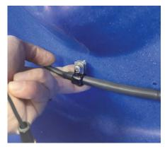
Attach the first clamp with one of the  $10/32 \times 3/4$ " bolts to hole A (hex nuts will be added later).
