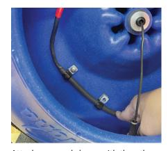
Attach a second clamp with the other  $10/32 \times 3/4$ " bolt to hole B.
