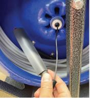
Slide the membrane sleeve over the push-rod connection.
