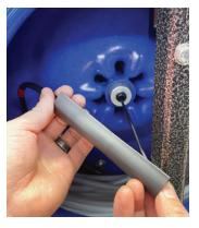
Position the membrane sleeve over both sides so the connection is covered completely.
