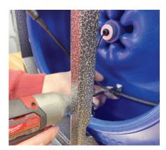
Screw in just until snug. You will tighten it completely after all the push-rod is loaded into the reel.
