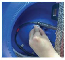
Line the clamps up with holes C and D and squeeze to tighten.
