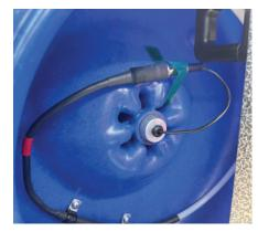
Put electrical tape over connection to keep it out of the way while feeding the rest of the push-rod into the reel.
