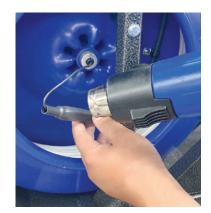
Use the heat gun to shrink the membrane over the connection.
