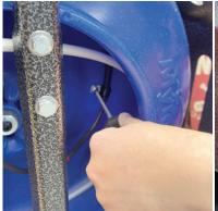
Hold the bolt secure on the inside as you tighten the nut on the backside using the 3/8" adapter on the power drill.
