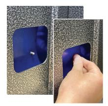
Screw the hex nuts onto the bolts on the back side of the reel, through the frame opening.
