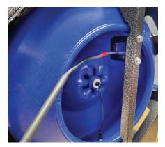
Feed the patch cord connection end of the new push-rod through the guide bracket so the push-rod will load in counter clockwise.
