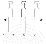
Peak & Null readings match From the Peak/Null location take several readings across cable. Mark position indicated by lowest depth reading. While stationary take multiple depth readings. Reading should be consistent
