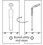
Maximum Null shows receiver signal line direction
