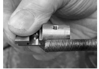
Set screws: 3 socket set, cup point, 8/32x1/8"
