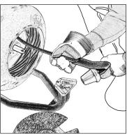
**2** Feed cable through the Revolving Arm tube. Fittings between the leader and main cable may need an extra push. **TAKE CARE** to not let the cable spring out of the reel
