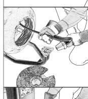
**4** Pull the cable out of the Revolving Arm and feed it completely back in to the reel
