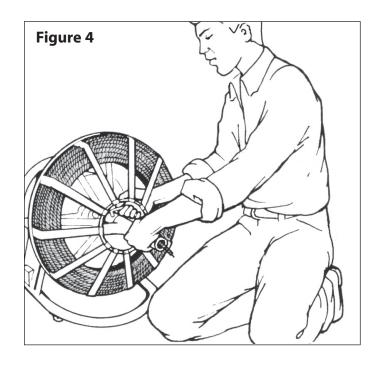
This combination revolving arm and cable is then placed on the part of the shaft protruding past the reel. Then, while holding the arm snug and secure against the, reel, tighten the set screw on arm securely to prevent slipping. (See Figure 4)
