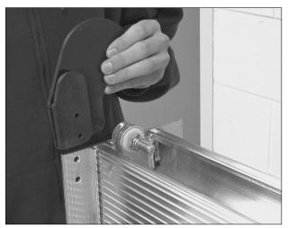
2. Lock the plastic covers in place with the hardware as shown. The female threaded grommet should be facing the ramp surface.
