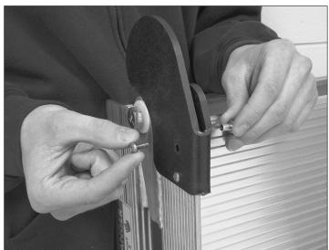
**3.** Using two philip screw drivers tighten the screws securely. You're ready to go!
