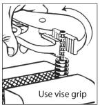
4. Clamp one cable end (pointing upward) in a bench vice, with the end of the cable 3/4" above the vice. Using a vice grip, screw half the core into the cable counter-clockwise.
