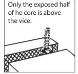
5. Now lower the same cable so the end will be even with the top of the vice, still pointing upward. Only the exposed half of the core should be above the vise. Then tighten the vice as much as possible. This will prevent the core from being unevenly divided when joining the other cable.
