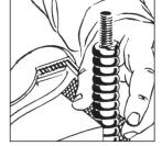
Same procedure applies on putting the core part of the male end in the cable (the end that cutting units are mounted on)
