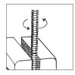
6. Join the other cable (counterclockwise) on the exposed half of the core and make sure that both ends of the cables fit tightly against each other.
