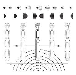
Trace the path by walking away from the transmitter at a moderate pace. Move the receiver to the left and right while walking, following the indications.
