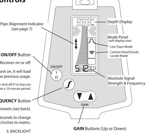
Use to adjust the gain level for the receiver. Continually adjust gain to high enough volume to hear. Also used to select CAMERA/SONDE or LINE mode (see page 2)
